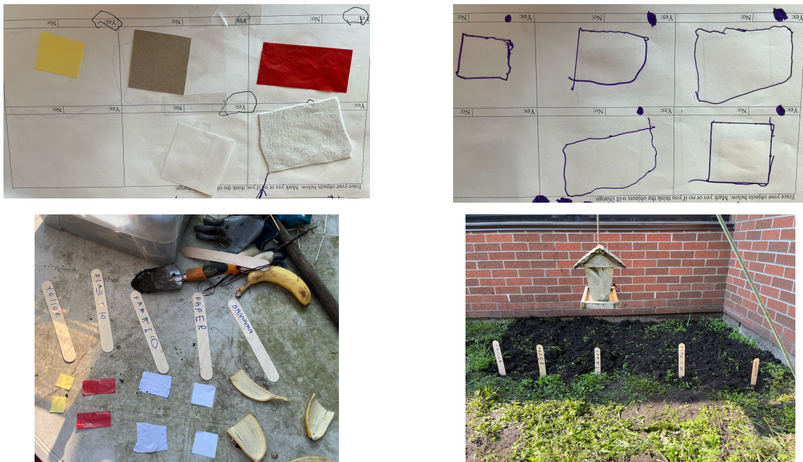
Figure 1: Objects glued or traced (top) and then buried in the soil (bottom).
